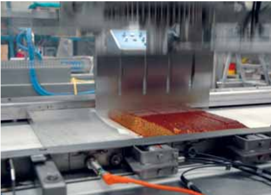
The secret is ultrasound, which makes the blade vibrate at 20,000 oscillations per second.
